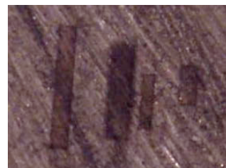
Fig. photo of exposed fluid inclusions in halite crystal
